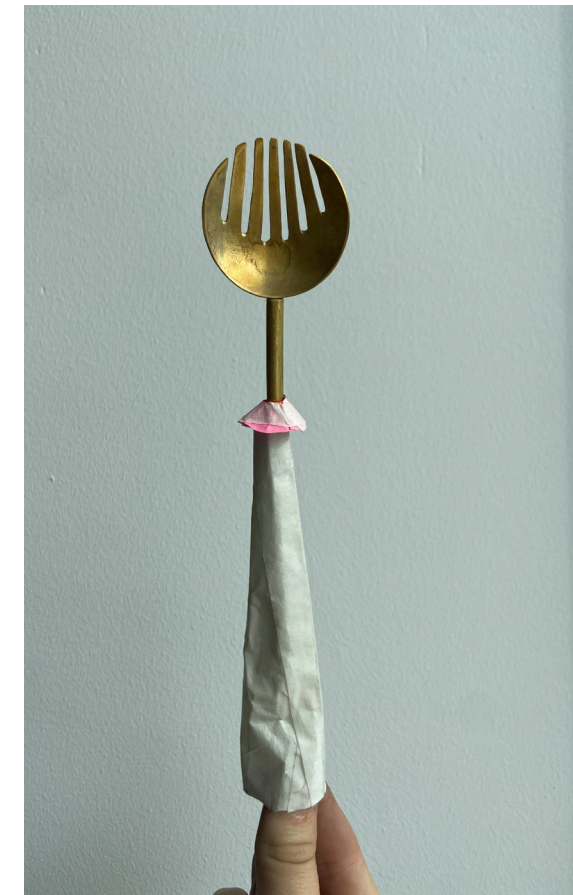
Brass parts, with mock up sleeve to analyse dimensions.
